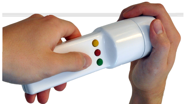
Figure 1. The Peppermill remote is an example of an interaction-powered interface device, which supports rotary input as the primary method of interaction.
