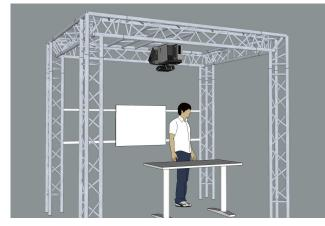
Figure 2: LightSpace configuration. All projectors and cameras are suspended at a central location above the users, leaving the rest of the space open and configurable.
