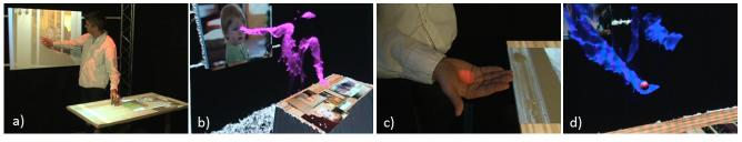
Figure 1: LightSpace prototype combines depth cameras and projectors to provide interactivity on and between surfaces in everyday environments. LightSpace interactions include through-body object transitions between existing interactive surfaces (a-b) and interactions with an object in hand (c-d). Images (a) and (c) show real images of the user experience, while images (b) and (d) show the virtual 3D mesh representation used to reason about users and interactions in space.
