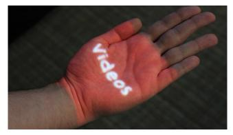
Figure 10: By aligning the projectors and the cameras, we can correctly project virtual content registered with the real world. In this case, we project a menu option directly onto the user's hand.
