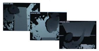
Figure 8: Raw depth images collected from three depth cameras each capturing a different part of the scene. Except where black, pixel intensity is proportional to the distance to camera (depth).
