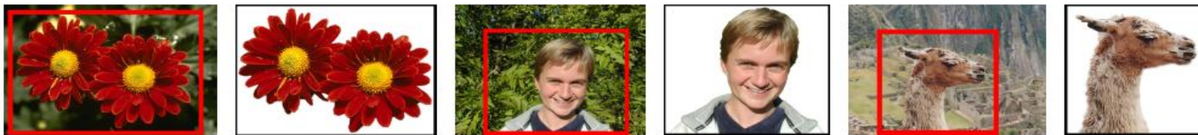
Figure 1: Three examples of GrabCut . The user drags a rectangle loosely around an object. The object is then extracted automatically.
