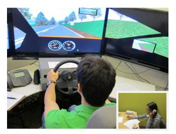
**Figure 1:** Participant driving the STISIM simulator. The simulator provides a console with speedometer, steering wheel with turn signals, and traditional brake and accelerator. Three 47" screens generate an impression of driving a vehicle. The driver used a speaker phone system (center left) to converse with the remote caller (inset).
