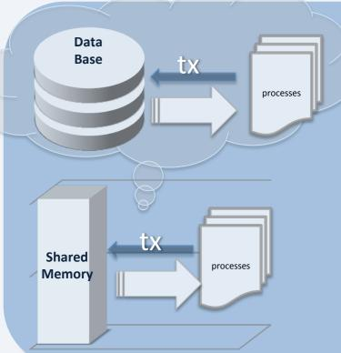
Transactional Memory (TM) adapts the concept of atomic accesses to multiple locations – a concept expressed through the transaction in databases for use in a multiprocess, shared memory system.
