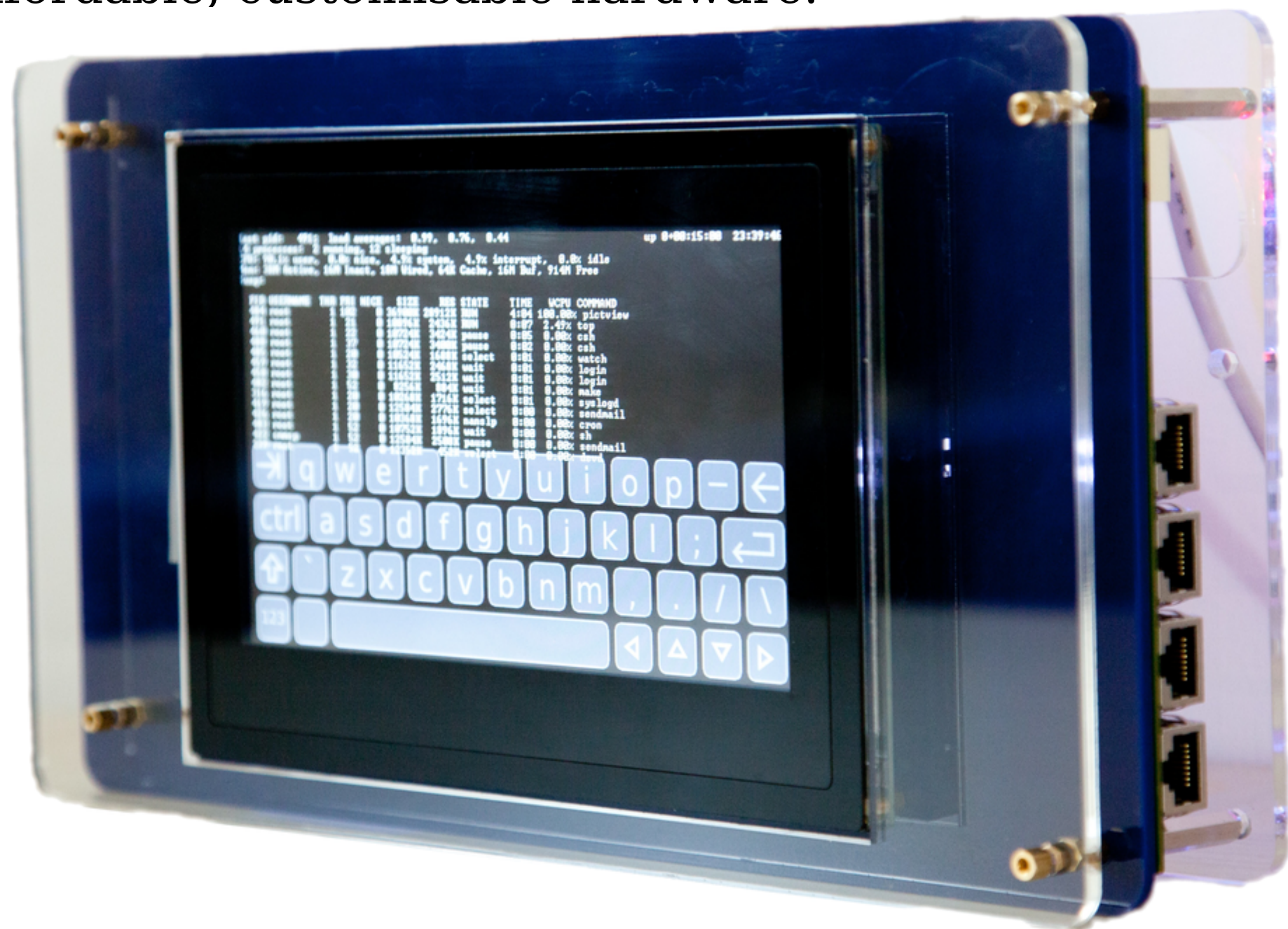
Figure 1: FreeBSD running on BERI on DE4 board
