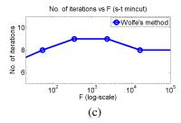
Figure 1: Running time comparision of Iwata-Orlin's (IO) method [11] vs Wolfe's method. (a): s-t mincut function, (b) Iwata's 3 groups function [16]. (c): Total number of iterations required by Wolfe's method for solving s-t mincut with increasing F
