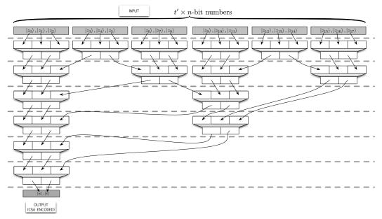
Fig. 12. Modular multiple addition of quantum integers on a CSA tile architecture for t' = 18 in a logarithmic-depth tree with height  $(\lceil \log_{\frac{3}{2}}(t'/3) \rceil + 1) = 6$ . Arrows represent teleportation in between modules.
