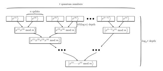
Fig. 13. Parallel modular exponentiation: multiplying t quantum integers in a  $O(\log(t) \log(n))$ -depth binary tree. Arrows indicate modular multiplication.
