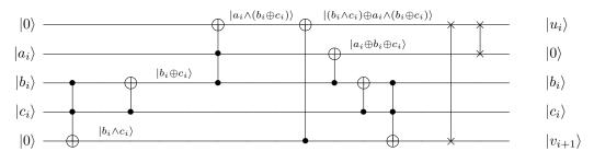
Fig. 6. Carry-save adder circuit for a single bit position *i*:  $a_i + b_i + c_i = u_i + v_{i+1}$ .
