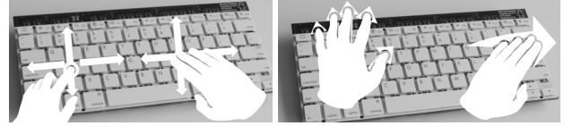
Figure 7. On-Keyboard swipe gestures. Gestures can be performed by either hand with single finger or whole hand.
