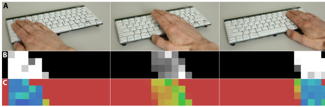
Figure 5. Sensor data. (A) Hand moving across the keyboard, including brief hover period (middle). (B) Sensor data is low-res but can be read at high frame rate (intensity encodes proximity). (C) False-color rendering, scale from blue (0mm) to red (400mm).
