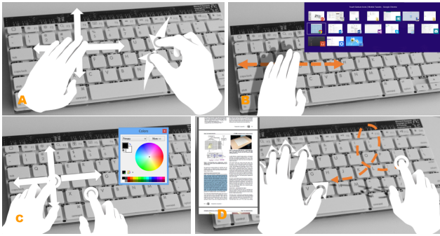
Figure 2. Usage scenarios. (A) Panning and Zooming a document. (B) Open hand hovering above keyboard invokes task switcher. (C) Pressing ‘C’ brings up color wheel and non-dominant hand selects color. (D) Coarse flicks scroll whole page; index finger performs a touch and hover ‘loop’ gesture to next/previous paragraph.
