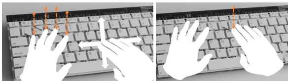
Figure 9. Micro-hover gestures. Hands remain in home position while typing or resting. Quick lifts off fingers triggers different commands.
