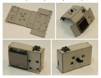
Figure 6. A cardboard digital camera case. Modules are mounted directly onto fold-out pillars and the unit fastens together in a 'tongue-and-groove' style; the display and pushbutton are external and everything else is internal.
