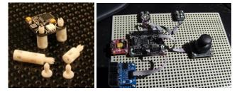
Figure 2. Perforated sheets can be used to secure electronic parts such as Gadgeteer. Left: Standard FR4 PCB sheet used with 3D printed end-stackable push-fit stand-offs. Right: A similar approach using off-the-shelf injection-molded plates and pop-rivets from Tamiya.
