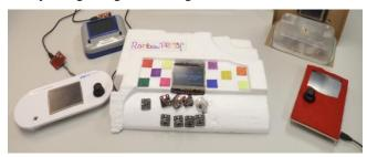
Figure 3. Prototype devices produced during a school pilot use a wide variety of materials to produce the required form-factors. These include (from left-to-right) printed cardboard, vacuum-formed plastic, expanded polystyrene, cardboard/plastic, and felt-over-cardboard.
