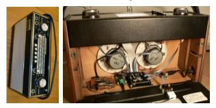
Figure 9. Retro-fitting an existing product is a great way to build a robust prototype with a very specific form factor. Here we show a Roberts radio which has been 'gutted' and retro-fitted with Gadgeteer modules.
