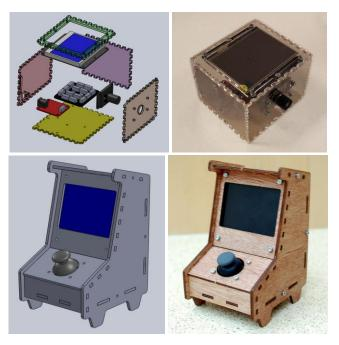
Figure 8. Bespoke enclosures created from laser-cut acrylic and plywood plates. 'Box Brownie' camera (top), mini arcade game (bottom). 3D models of the Gadgeteer modules are used (left) to ensure perfect fit (right).
