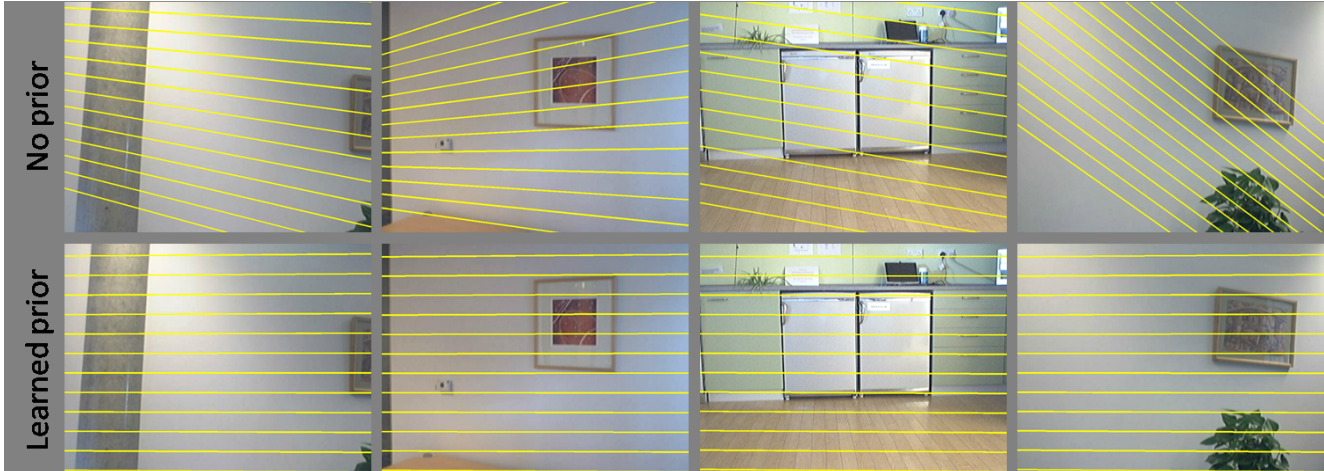
Figure 1. Stereo camera calibration results in typical structure-poor scenes. Four image pairs were obtained by a single stereo camera (only right-eye views are shown) and stereo correspondences were obtained by robust feature matching. Without a prior, standard camera calibration techniques fail and the recovered epipolar geometry (shown using epipolar lines) is inaccurate (top row). By using a prior learned by the method described in this paper, accurate (and consistent) calibration is obtained (bottom row).
