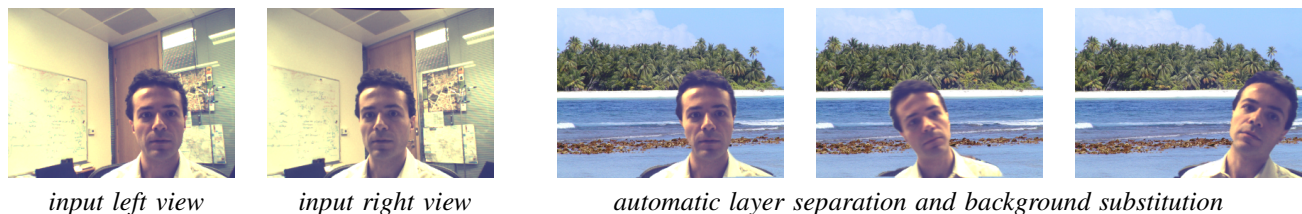
Fig. 1. An example of automatic foreground/background separation in binocular stereo sequences. The extracted foreground sequence can be composited free of aliasing with different static or moving backgrounds; a useful tool in video-conferencing applications. Stereo sequence AC used here. Note: the input synchronized stereo sequences used throughout this paper can be downloaded from [1], together with hand-labeled segmentations.
