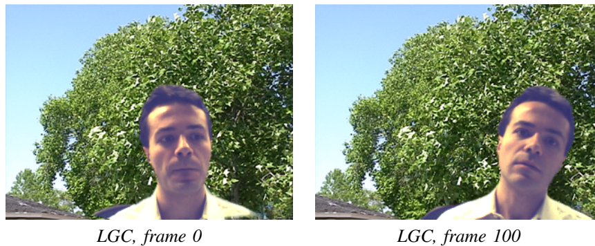
Fig. 10. Segmentation and background substitution. Here we show background substitution (using LGC) for two frames of the sequence AC.
