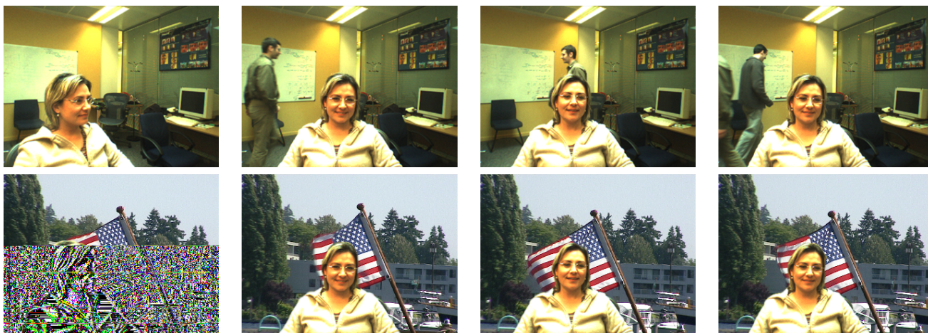
Fig. 11. Segmentation with non-stationary background. (Top) Four frames of the input left sequence IU (right frame not shown here). (Bottom) Corresponding LGC segmentation and background substitution. LDP performs similarly. Note the robustness of the segmentation to motion in the original background.
