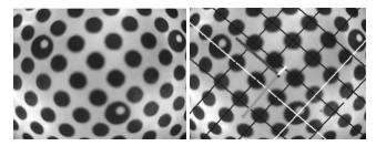
Fig. 3 *Left*. Raw input image showing the 2D grid pattern. *Right*. Vision algorithm extraction of grid orientation.
