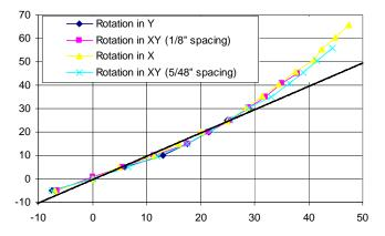
Fig. 5 Actual angle vs. computed angle for the vision tracker. The dotted line shows the ideal response. Angle estimates are fairly accurate between the -20° and 20° range used in practice. Estimates are consistent over different grid orientations and spacings
