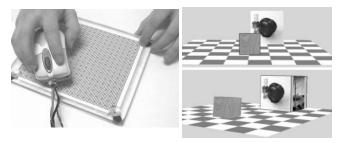
Fig. 6 Two-handed rotation of the mouse pad allows rotation of the entire scene. To resolve the depth ambiguity seen here in the top right image, the user has rotated the ground plane to a different viewpoint (bottom right).
