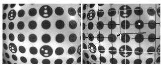
*Fig. 4* The revised grid encodes position information in the large dots for better tracking of rapid 2D mouse motions.
