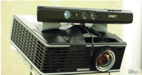
Figure 3. The Juggling Display pro-cam unit consisting of InFocus IN1503 projector and a Kinect for Windows camera.
