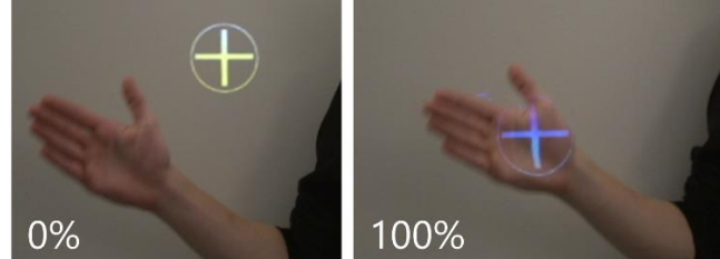
Figure 5. Image showing projection slip on fast human motion under no prediction and alignment under full latency prediction with memory lookup approach.
