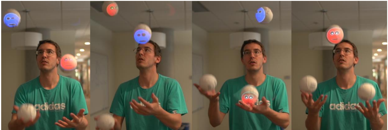
Figure 1. The Juggling Display is a custom projector-camera system demonstrating our motion prediction strategies for reducing the effects of latency on projection alignment. Through prediction, our system improves target illumination by 30%.
