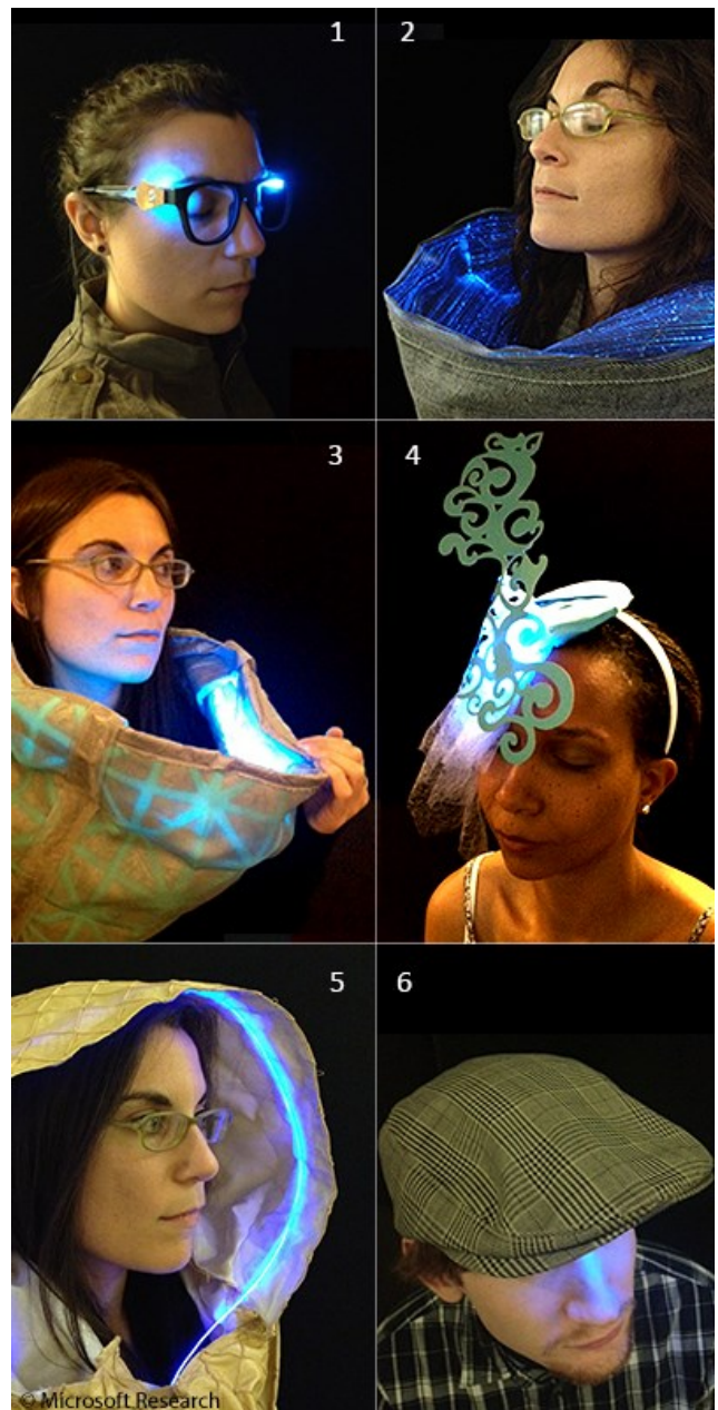
Figure 5. Wearable light-emitting prototypes – Glasses (1), Fiber Optic Scarf (2), Teal Cowl (3), Fascinator Hat (4), Hood (5), and Classic Golfer’s Hat (6).
