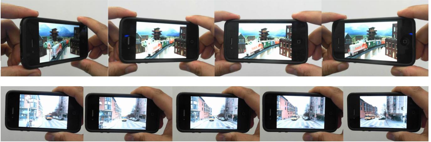
Figure 6. Frames depicting the changes in parallax as the viewer manipulates the device.
