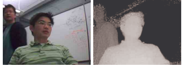
Fig. 4. Sample output from ZCam [2] (left: color image; right: depth image).
