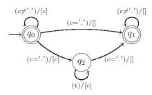
**Figure 5:** Symbolic finite state transducer for uptoLast(c=`.', input). This transducer is non-deterministic; there are two transitions that match `.' from state  $q_0$ .
