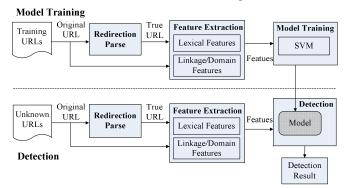
Figure 1. The flowchart of our detection system
