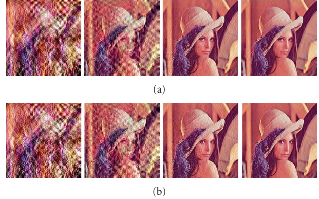
FIGURE 10: Rendered images for unencrypted (a) and encrypted (b) “Lena” for bit error rates of 0.00005, 0.0001, 0.001, and 0.01.
