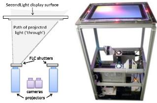
Figure 10: The layout of the main SecondLight components. On the left we show a cross-section through the side of the unit (this is during the 'through' phase when the second projector is active and light from the on surface projector is blocked). The far left is the front of the unit and thus the through projection is angled away from the user. On the right is a photo of the unit taken from the front.
