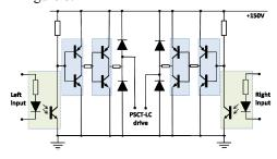
Figure 9: The PSCT-LC H-bridge driver circuit.
