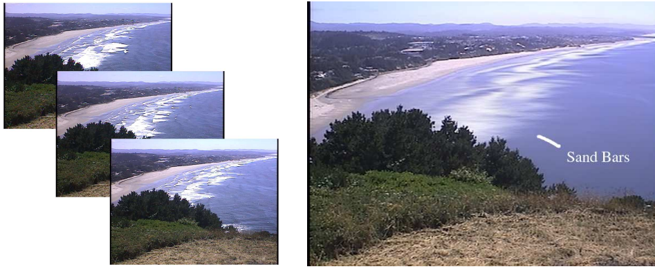
Figure 3.6: Images from the IrisNet Coastal Imaging prototype. On the left, raw video frames. On the right, temporally smoothed images revealing the sand bars.
