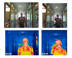
**Figure 4:** RGB images (top) vs. FIR images (botton): The image on the right shows that a off-the-record gesture (trying to block the camera) can be also detected using an FIR image.
