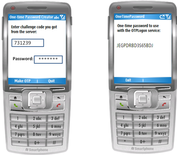
Fig. 2. The application was implemented on a Windows Mobile 6.0 smartphone simulator and then ported to a BenQ E72 smart-phone. The figure depicts the simulator screenshot. The application running on the device accepts the input nonce N and produces the output code E(p, h(K_d, N)) . Figure shows the device after user has entered N (left) and after the output code E(p, h(K_d, N)) has been generated (right). The user will enter the latter at the untrusted terminal.
