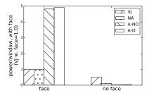
Figure 3: Impact of gating on power consumption.
