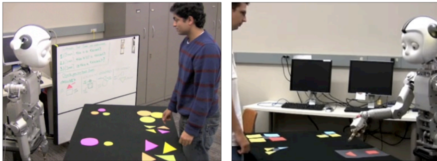
Figure 3: Users teaching new concepts to a robot by providing positive and negative examples. (Left) Passive learning: examples are chosen and presented by the user. (Right) Active learning: particular examples are requested by the learner. Although active learning results in faster convergence, users get frustrated from having to answer the learner's long stream of questions and not having control over the interaction.
