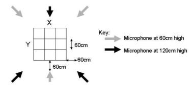
Fig. 6. Experiment setup for 3D experiments
