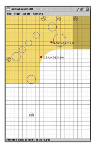
**Fig. 9.** GUI for configuring audio location and defining 3D user interfaces. A plan view of an office room with a corner desk is used for the background. The concentric circles represent microphones, the large unshaded circles represent buttons, and the small shaded circles represent finger clicks recently detected, along with their coordinates. Of the six microphones in the prototype, one is off the side of this plot and therefore not shown.
