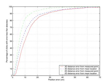
Fig. 7. Cumulative frequency plot of location error measurements
