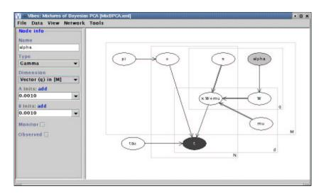
Figure 2: Screen shot from VIBES showing the graph for a mixture of probabilistic PCA distributions. The node t is coloured black to denote that this variable is observed, and the node 'alpha' has been highlighted and its properties (e.g. the form of the distribution) can be changed using the menus on the left hand side. The node labelled 'x.W+mu' is a deterministic node, and the double arrows denote deterministic relationships.
