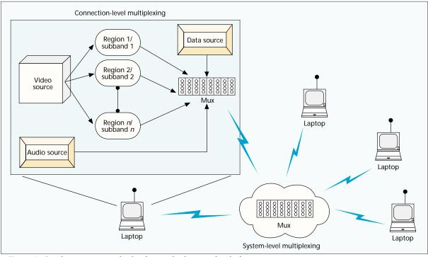
Figure 5. Comibining connection-level and system-level statistical multiplexing.
