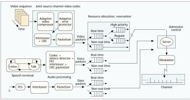
Figure 3. Conceptual model for a video-capable wireless device.
