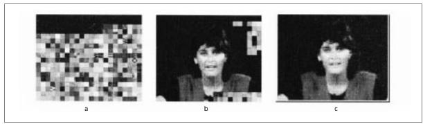
■ Figure 4. Alleviating error propagation with spatial and frequency decomposition: a) bitstream corruption of the Miss America sequence in ITU's H.263; b) after region segmentation; c) iafter region segmentation, frequency segmentation, and prioritized transmission (PSNR: 3.2.34 dB).
