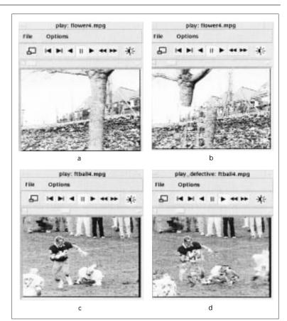
Figure 1. The effect of temporal and spatial error propagation in current ISO and ITU video codecs: a) frame #16; b) frame #31; c) original; d) with spatial error propagation.
