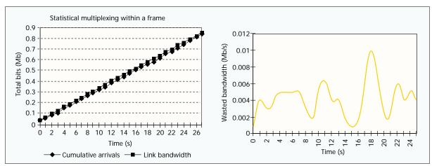
Figure 6. Intraframe statistical multiplexing for a region-segmented video codec.
