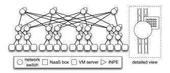
Figure 1: NaaS architecture in a data centre.
