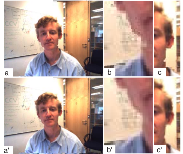
Figure 10: A two-camera video-conferencing example. (a) Cyclopean view after first pass. The two input images are not shown here. (b,c) Details of (a) showing aliasing artefacts along the head boundary. (a') Cyclopean view after SPS enhancement. (b',c') Details of (a') where the introduction of pixel mixing produces an enhanced outline of the foreground object.
