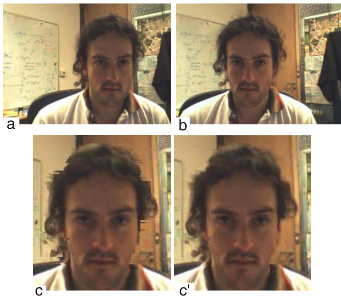
Figure 1: High-quality two-camera virtual-view synthesis. (a,b) Left and right input images (size 320 \times 240 ) with large disparities and occlusions (60 pixel max disparity). (c) Virtual cyclopean image (detail) recovered by a standard dense stereo algorithm [7]. Along the boundary of the head streaky and blocky artefacts and aliasing effects occur. (c') Virtual cyclopean image (detail) after the proposed SPS enhancement step. The removal of artefacts and the introduction of mixed pixels produce a more natural-looking synthetic image.
