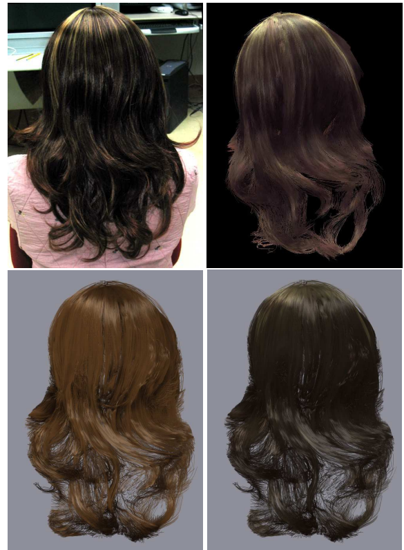
Figure 6: Example of a typical long wavy hair style. One of the original images on the top left. The recovered hair rendered with recovered diffuse colors on the top right, rendered with a constant hair color using the self-shadowing algorithm on the bottom left, rendered with the recovered diffuse colors using the self-shadowing algorithm on the bottom right.
