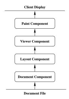
Figure 7: Simplified composition of the word-processing components.
