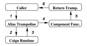
Figure 4: Calling sequence for first call to an aliased function without IDL information. Control passes from caller to trampoline function (1) then into the Coign runtime (2). The runtime returns a special value to the trampoline (3) which patches the stack. Control jumps directly into the component function (4) which returns to another trampoline (5) and then jumps back into the caller (6).
