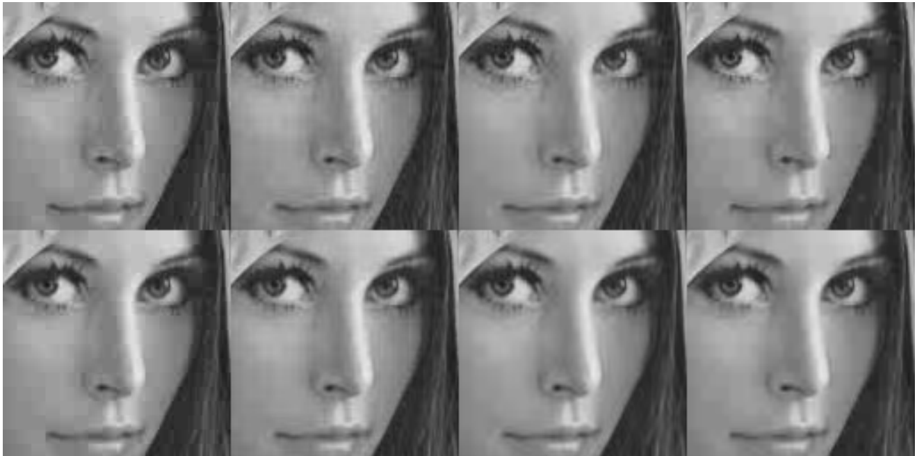
Figure 5: Coding examples for image "lena2" at 0.6 bits/pixel. Top row: JPEG encoding; column order, left to right: DCT, LOT, LBT, HLBT, with PSNR (dB) = 33.0, 33.3, 33.7, and 33.4, respectively. Bottom row: embedded zerotree encoding; column order, left to right: DCT, LOT, LBT, HLBT, with PSNR (dB) = 34.0, 34.5, 34.9, and 34.5.
