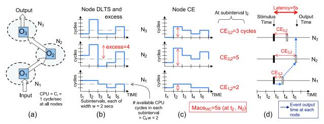
Fig. 3. (a) An example CQ plan on 3 nodes. (b) DLTS for each of the nodes, over 5 subintervals. Here, subinterval width is w = 2 secs and CPU on each node is  $C_i = 1$  cycle/sec. (c) CE for each of the nodes, with CE at subinterval  $t_2$  highlighted. Worst-case CE (Mace<sub>WC</sub>) is shown. (d) Lifetime of an event *e* which enters EPS at the end of subinterval  $t_2$ . Latency of  $e = Mace_{WC} = 5$  secs.
