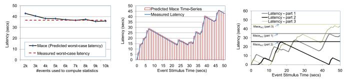
Fig. 4. Estimated vs. actual Lat<sub>WC</sub>, increasing Fig. 5. Latency and Mace for the entire time-series. Fig. 6. Latency and Mace<sub>WC</sub> for different data training size.
