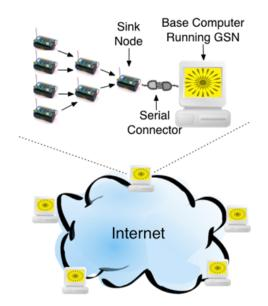
Fig. 1. A standard application of GSN (top) showing GSN gathering data from a sensor network via a serial forwarder that is itself connected to the network's sink node. GSN also offers the functionality of connecting several GSN instances to allow advanced query processing.
