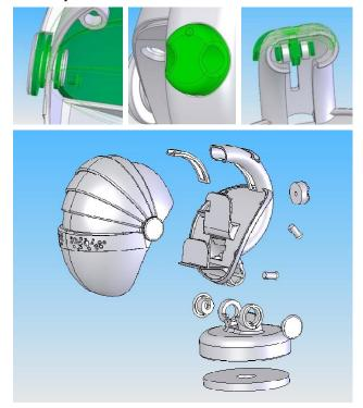
Fig. 11. The 3D modelled additional features and an exploded view of all the separate components.
