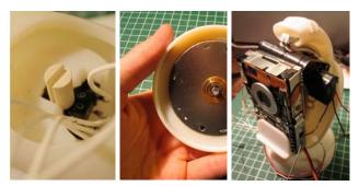
Fig. 12. The integration of the electronics in the printed parts.
