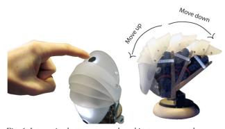
Fig. 6. Interactive buttons; tap makes object move up or down.
