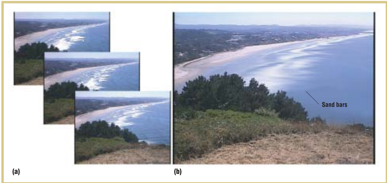
Figure 8. Coastal images in the form of (a) raw video frames and (b) 10-minute time-averaged exposure.
