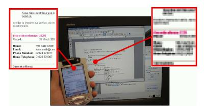
Fig. 2. Our prototype in use. Content on the public terminal is censored (right inset); the area around the mouse pointer appears uncensored on the private display (left inset). In this case, pixellation is used for censoring the public display, but other filters are also provided.
