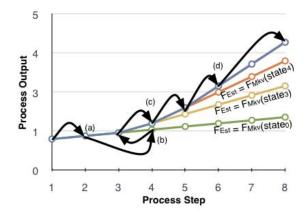
Figure 4: An example execution of the Markov Jump algorithm. The algorithm starts by performing a fingerprint-sized sampling (a) from the markov chain, until the fingerprint differs from a synthesized estimator (b), then backtracks and synthesizes a new estimator (c). This process repeats until it finds an estimator valid for the remainder of the chain (d).
