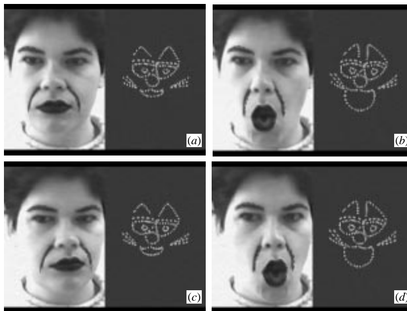
Figure 4. Pose-invariant transmission of facial expression. Separation of non-rigid from rigid motion by SVD is used here to extract the facial expression of an actor. The extracted expression is displayed on this cat caricature in a fixed pose, and can be seen to be independent of the pose of the actor's head.
