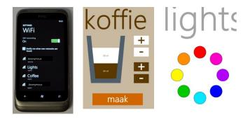
Figure 2. To access a SAWUI, a user chooses the appliance from the WiFi settings screen (left) of their phone. The SAWUI automatically appears with no further user input. We prototyped a SAWUI-controlled coffee machine (middle) and mood light (right). The phone's language setting is used automatically. Cookies store personal settings persistently.
