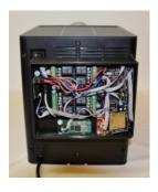
(d) Rear of coffee machine showing prototyping electronics
