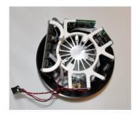
(b) Inside of mood light showing AP module (top) and other prototyping electronics
