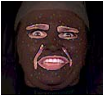
Figure 9: Masks surrounding important facial features. The gradient of a blurred version of this mask is used to orient the low-pass filters used in the dot removal process.
