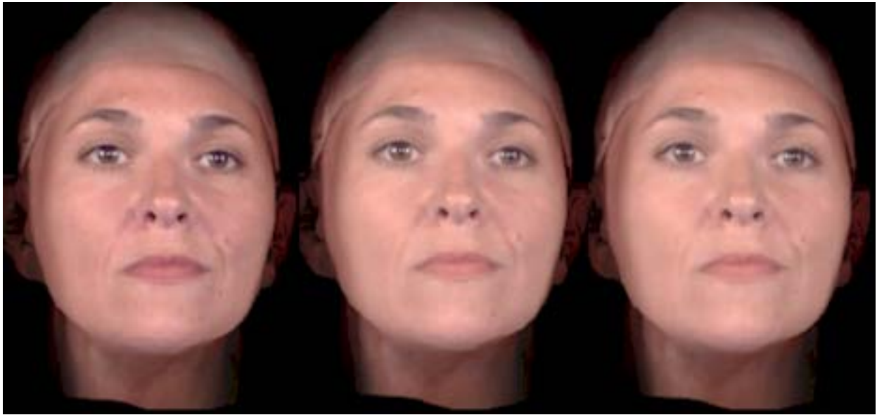
Figure 14: Left to Right: Mesh with uncompressed textures, compressed to 400 kbits/sec, and compressed to 200 kbits/sec
