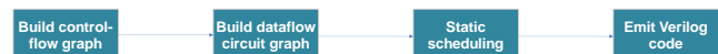
Figure 2: The four passes of M2V, a compiler that translates MIPS instruction sequences into circuits.
