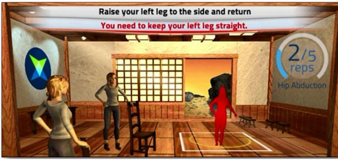
(a) A physical therapy application from Reflexion Health. The application senses the user’s position using a Kinect sensor. On the right, the application displays a visualization of the user’s current position. Along the top, the application describes the gesture the user must perform in English. The application also provides feedback to the user on how to better perform the gesture.
