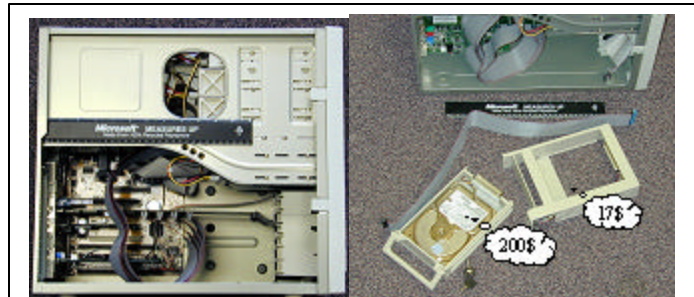
Figure 5: Inexpensive terabytes. A no-name PC includes a 700Mhz processor, 256MB ram, gigabit Ethernet, and housing for 8 disks. This costs 1k$ for the computer and 2k$ for the disks (and controller). The net is 7K$ per TB. The disks are hot- pluggable. They can be used for data interchange or for backup, eliminating the need for tape.
