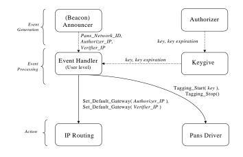
Figure 3: Architecture for auto-configuration of PANS
