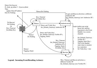
Figure 4: State Transition Diagram for the Event Handler
