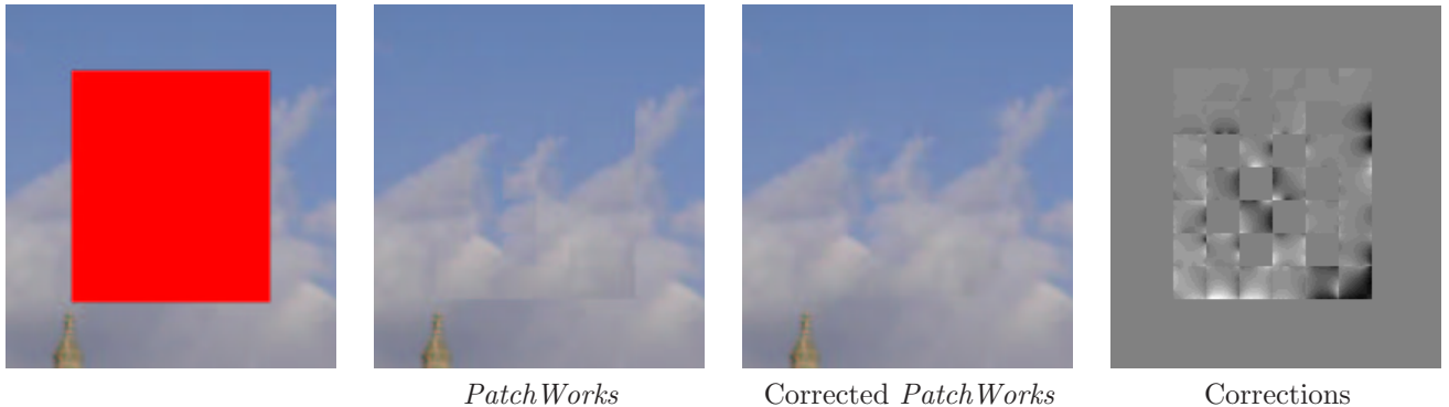
Fig 20. Removing seams by post-processing. The tiling obtained with a small dictionary of 20 \times 20 blocks exhibits a few visible seams in this example. These seams are removed by applying an appropriate smooth additive correction to all the patches of the first inner layer, and to every other patch on the other layers. The corrections shown on the right are those applied in the green color channel. [size of destination region: 140 \times 120 pixels; w = 20 , p = 2 , \ell = 40 .]
