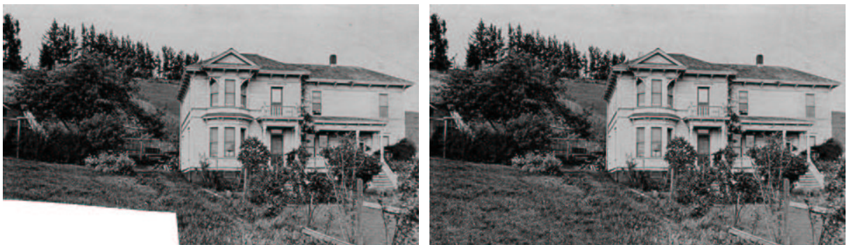
Fig 13. Completing old photographs. It is quite common for old photographs to have torn borders. After digitization, PatchWorks can be used to re-invent the missing parts. On this 276 \times 476 digitized old photograph, the 8,200 missing pixels in the lower left corner were filled in 0.2s. After 2min45s, Resynthesizer filled the same area in a much less satisfactory way, with artifacts appearing in the grass.
