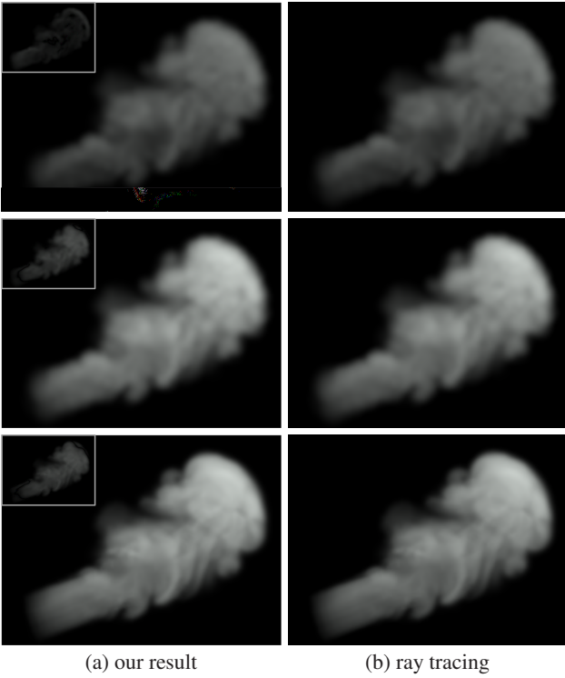
Figure 6: Comparison between our results and ray tracing. Top: single scattering in an approximated density field (root mean square (RMS) error:4.3%). Middle: single and multiple scattering in the approximated density field (RMS error:13.8%). Bottom: final results for the original density field (RMS error:14.1%). Lighting comes mainly from the top-right corner. The ray tracing result takes 47 minutes to compute, while ours renders at real-time rates. The smoke density ranges from 0.0 to 1.1, \sigma_t = 2.49 , \Omega = 0.66 , and the smoke volume width is about 3.0 meters. Absolute differences are included as insets.
