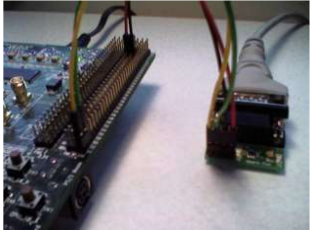
Figure 8: Cabling for the ML401 Board
